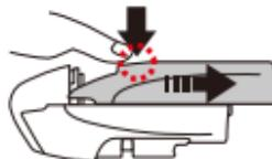
Remove top body by pushing down while sliding it backward.
