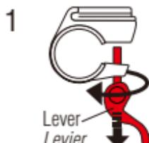
Attach the bracket to the handle bar securely. Place the rubber pad in the bracket to keep the bracket from rattling.
