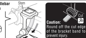
When attaching the bracket to the handlebar
