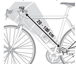
**B** The magnet faces the sensor zone of the sensor.
