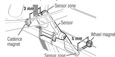
\* The wheel magnet may be installed anywhere on the spoke if the above installation conditions are satisfied.
