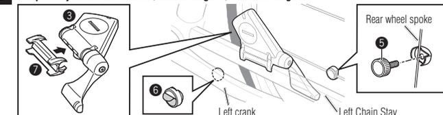
\* Temporarily install the sensor and 2 magnets at the respective points that satisfy the condition **B**. When the condition cannot be satisfied, move the sensor in the front-and-rear direction to adjust.
