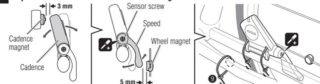
\* Loosen the sensor screw to adjust the speed. After adjustment, firmly tighten the sensor screw and nylon tie to fix.
