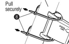
\* Install the sensor as close to the upper part of the front fork as possible.
