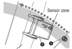
**C** The clearance between the sensor surface and the magnet must not exceed 5 mm.
