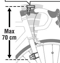
**B** The magnet must pass through the sensor zone.
